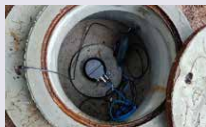
INSTALLED CERTIMUS SEISMOMETER CREDIT: DR. PHILIP HERING, GOETHE-UNIVERSITY FRANKFURT
