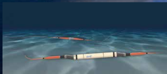
ILLUSTRATION OF THE CABLED REPEATER AND INLINE INSTRUMENT POD ON THE SEAFLOOR
