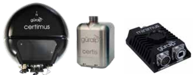
LEFT TO RIGHT: GÜRALP'S CERTIMUS DIGITAL SEISMOMETER, CERTIS SEISMOMETER AND MINIMUS DIGITISER
