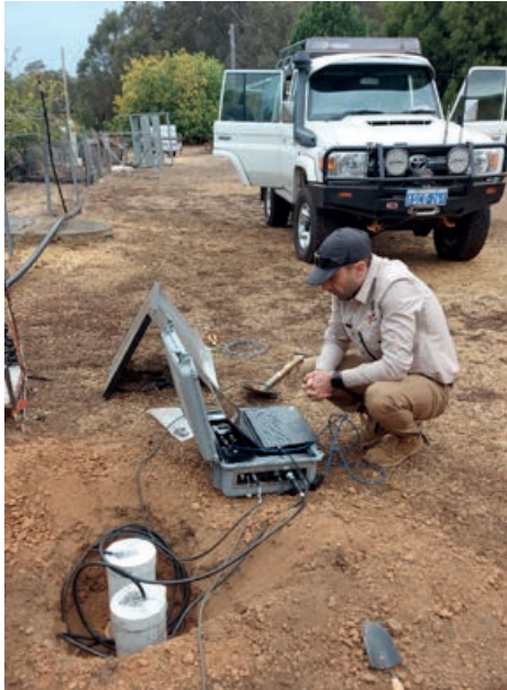
Figure 2: Reza Ebrahimi of GSWA installing the Güralp rapid deployment kit in the Perth Hills
