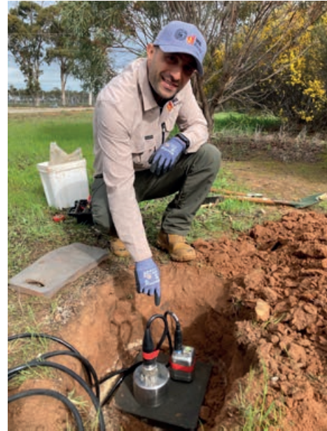
Figure 3: The Certis and Fortis-PH being deployed in a pit in the Wyalkatchem region of the Wheatbelt of WA
