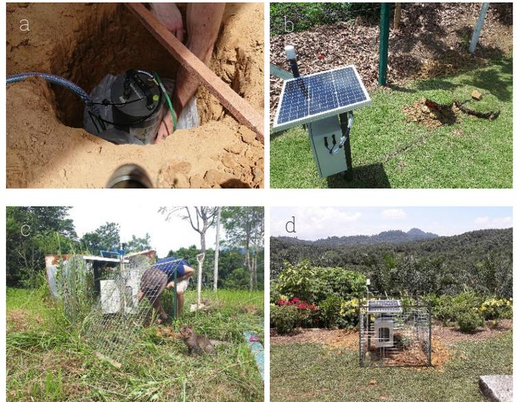
Figure 5: Clockwise from top left: (a) installation of seismometer (b) solar powered transmitter (c) housing installation featuring local feline (d) completed station.
