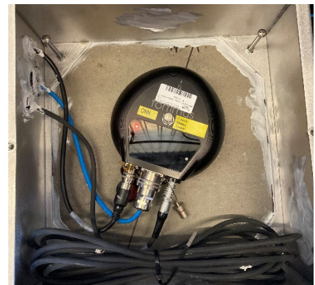
Figure 3: Sensor placed in vault and cabled in.
