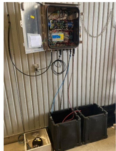
Figure 4: Control box for battery power supply and modems. Black boxes below contain batteries to power the sensor.
