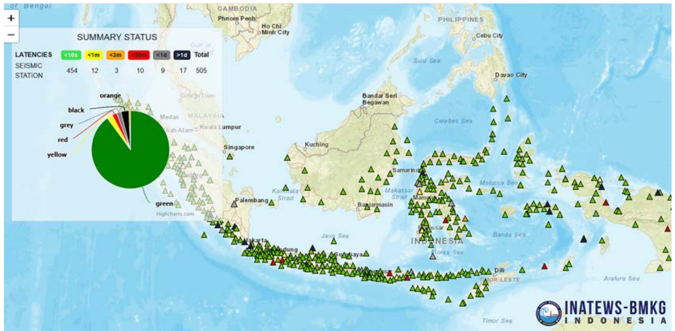
Figure 1. A still from the SeedLink monitor showing realtime seismic stations
