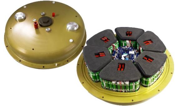
Figure 2 Aquarius pressure vessel showing internal sensors, digitiser and battery packs
