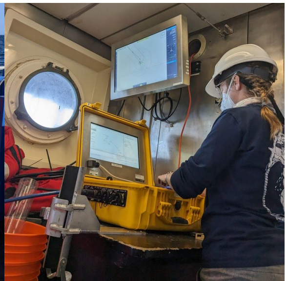
Figure 5. Acoustic communication through the deck unit to an underwater instrument. Photo courtesy of John Thibodeau.
