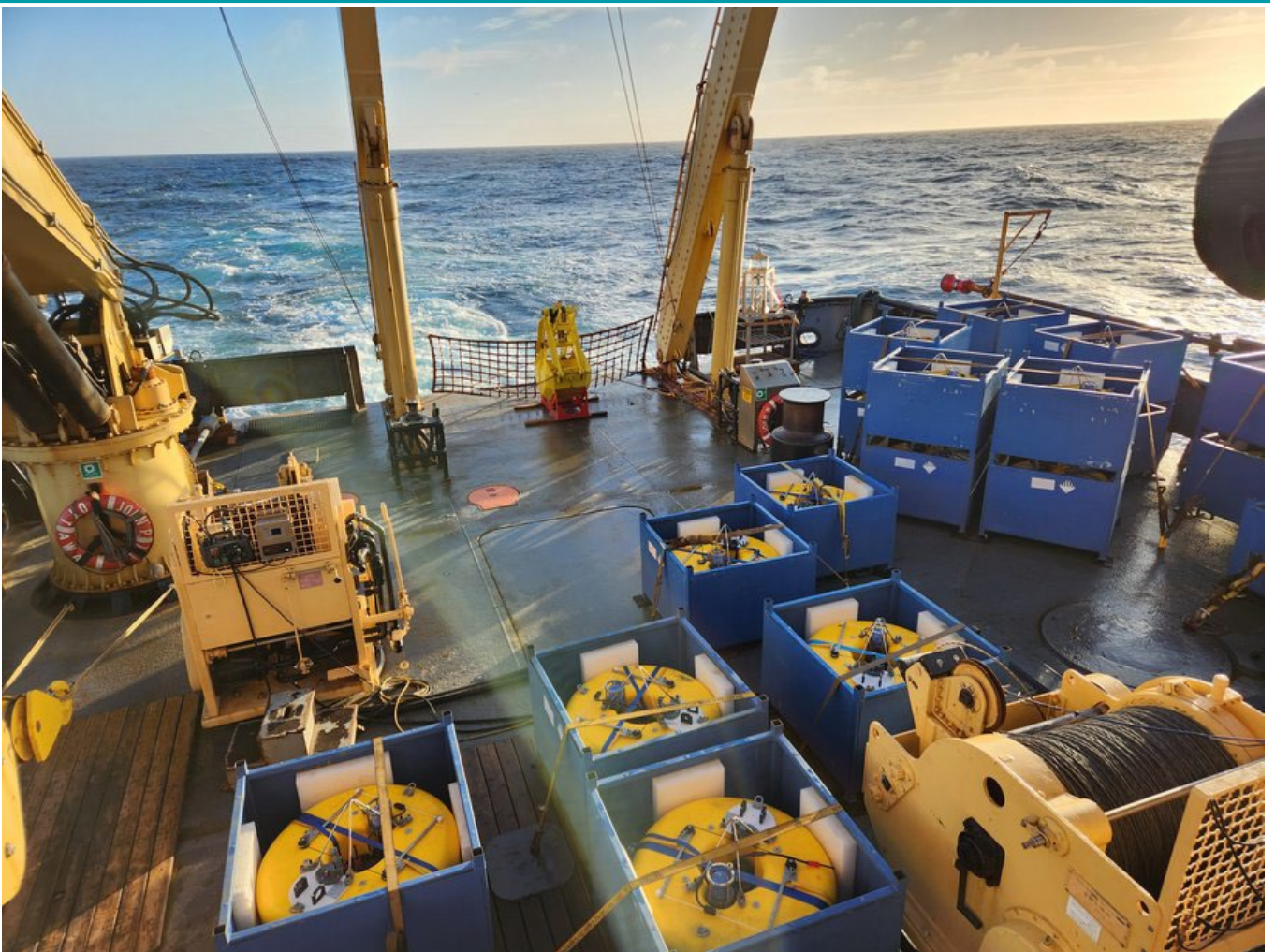
Figure 1. Güralp Aquarius OBS on route to Vancouver Island. Photo courtesy of Katie Bosman
