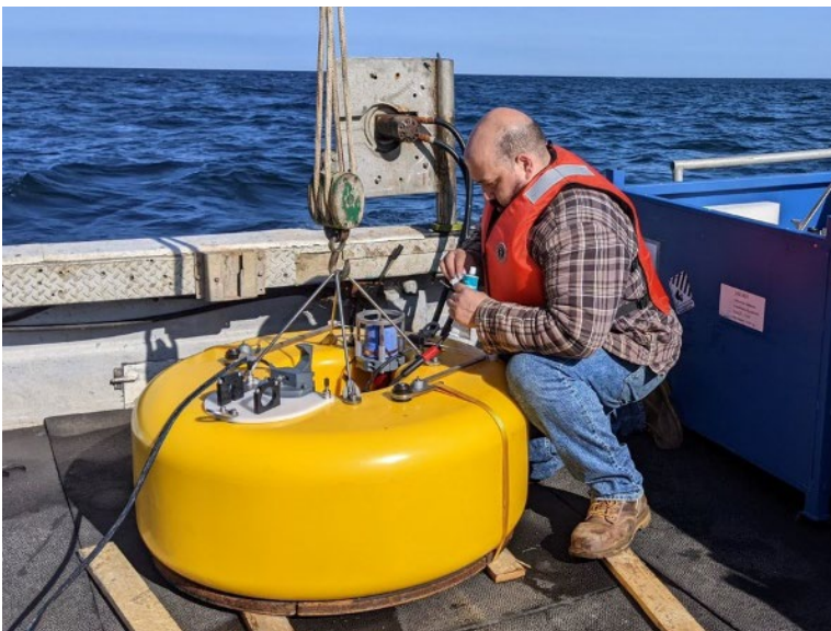
Figure 4. John Thibodeau checking electrical connections on the Aquarius prior to deployment. Photo courtesy of Katie Bosman
