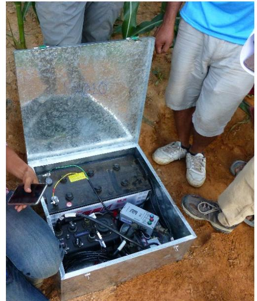
Figure 3. An 'Action Packer' – Digitizer, breakout box, battery and power box.
