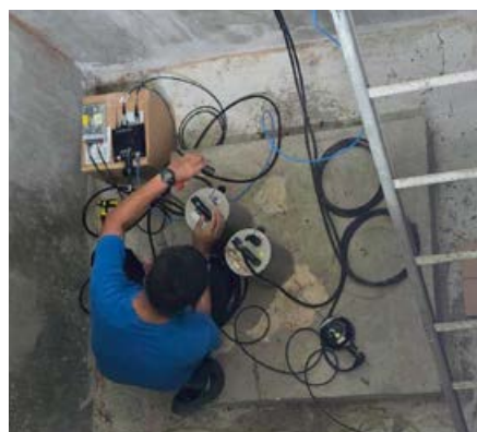
Figure 16 (left): A 3T deployment in a dedicated vault enclosure onto a concrete plinth installed onto bedrock.
