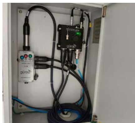
Figure 16 (left): A 3T deployment in a dedicated vault enclosure onto a concrete plinth installed onto bedrock.
